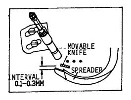
WHEN MOVEABLE KNIFE MOVE FORWARD AND MEET WITH SPREADER, THE TIP OF HOOK BLADE SHOULD SQUARE MATCH TO THE THREAD HOOK OF SPREADER. LOOSEN THE SET SCREW, ADJUST THE HOOK BLADE OF MOVABLE KNIFE TO ITS PROPER POSITION AND LINE UP WITH THREAD HOOK OF SPREADER THEN TIGHTEN THE SET SCREW.
